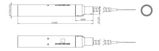
• Collimator with isolator. 4mm diameter beam M2<1.2
